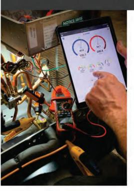
measureQuick (mQ) is an app that collects and analyzes heating and cooling system performance using Bluetooth®
